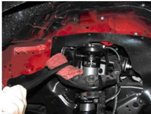
7. Install new coil assembly: there are 6 threaded holes in the top of the upper shock mount. You will be using 3 of them, the holes with a dot next to them are for Tacoma and 4runner, and the holes without a dot are for Tundra and Sequoia. Install upper mount with the charge port pointing outward using (3) 3/8" bolts and lock washers.
